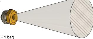
\*(air pressure = 2 bar, pressure medium = 1 bar) flow rate at 1 bar: approx. 0,65ml/sec (using water)
