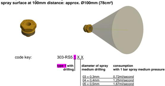
to achieve a reduced consumption with large internal cross-section this replace nozzle has a restrictor:
